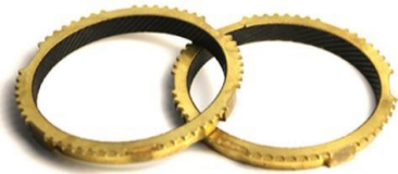
Carbon fiber friction brass rings
